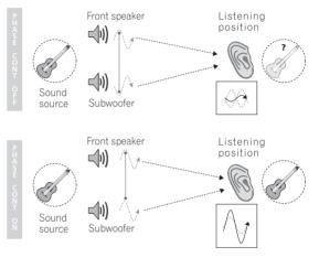
Phase Control technology provides coherent sound reproduction through the use of phase matching<sup>4</sup> for an optimal sound image at your listening position. The default setting is on and we recommend leaving Phase Control switched on for all sound sources.
